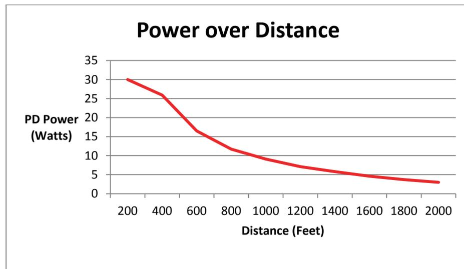
Figure 1: Transition Networks [Ethernet Over Coax Extender With PoE+](#) Power versus Distance Performance\*
