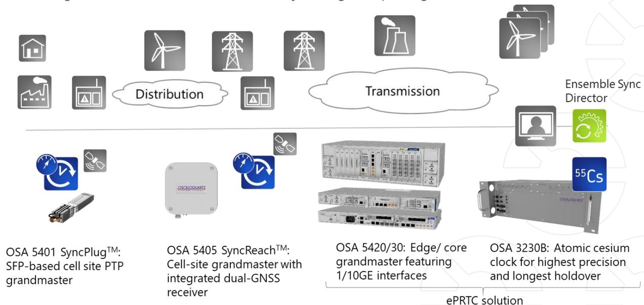
The OSA 5420 is an essential component for timing excellence at power networks. It supports the widest range of interfaces. The OSA 5420 is concurrently supporting multiple PTP profiles and can favorably be applied as a gateway between telecom and enterprise timing networks.
