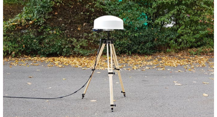
Fig. 4. Tripod – Short-term local DF operation, quick and easy to install
