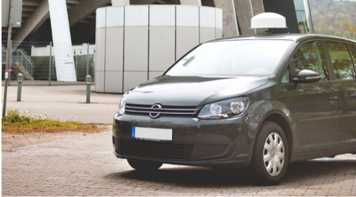
Fig. 3. Magnetic mount - Non-destructive, fast mounting on a vehicle roof
